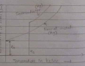
of a normal metal silver (Ag) and a superconducting metal mercury (Hg) versus temperature.
