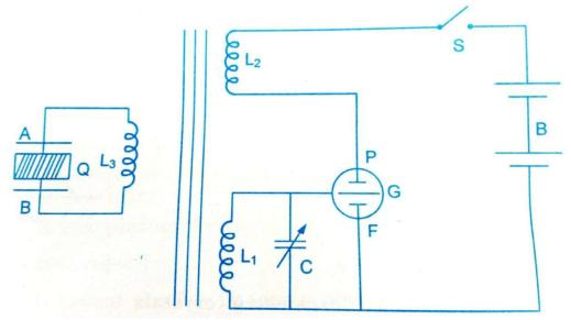
The experimental arrangement is shown in fig. Quartz crystal Q is placed between two metal plates A and B, connected to the coil  $L_3$ . The coil  $L_1$ ,  $L_2$  and  $L_3$  is connected to triode valve. Coil  $L_1$  is connected parallel with variable capacitor  $C_1$  forming the tank circuit. The high tension battery is connected between free end of  $L_2$  and the cathode of triode.
