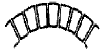
bricks cut to a wedge shape and mortar joints of uniform thickness
