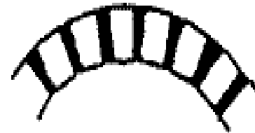
uncut bricks with wedge shaped mortar joints
