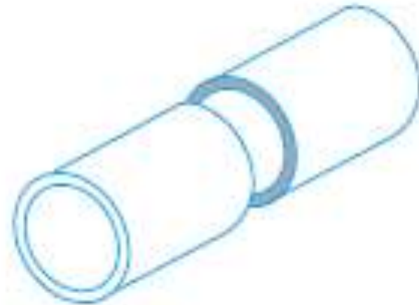
(b) Failure of a cylindrical shell along the transverse section.
